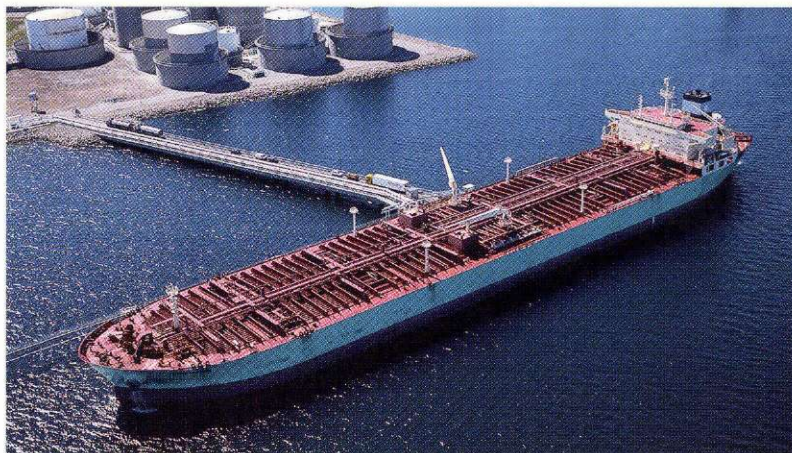
PETER MÆRSK on a rare visit to Copenhagen in 2001. The vessel is a modern double-hull, coated Aframax tanker of 110,000 dwt, delivered from Dalian in 1999.
