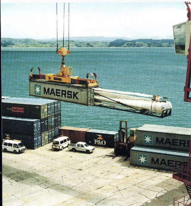
The 23.5 m long sails represent one of the longest out of gauge cargoes to be carried by Maersk Line.
